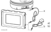
Power supply cable from 3D Disto Power supply from mains supply with AC/DC adapter
