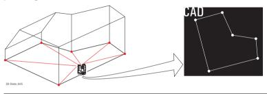
Layout orDesign data in DXF format can be imported and used to lay out the correspondingprojectionpoints or grids.
