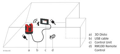
3D Disto is operated by the Control Unit. Certain functions can also be executed using the RM100 Remote Control.
