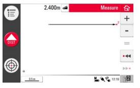
6. After the third point is measured a proposed "closing line" appears between the first and last measured point. The selected line is always highlighted with a bold line and an arrow in the direction of measurement.
