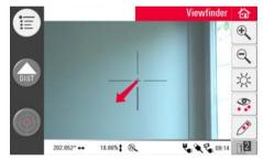
3. Press or to zoom in and out. There are four magnifications available. The current setting is shown in the status bar.
