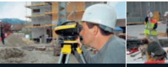
Elevation control, height control Platform/concrete casting stakeout, rectangular area stakeout, distance measuring As-built elevation checking, grade checking, area levelling, volume determination of earth/dirt moving operations
